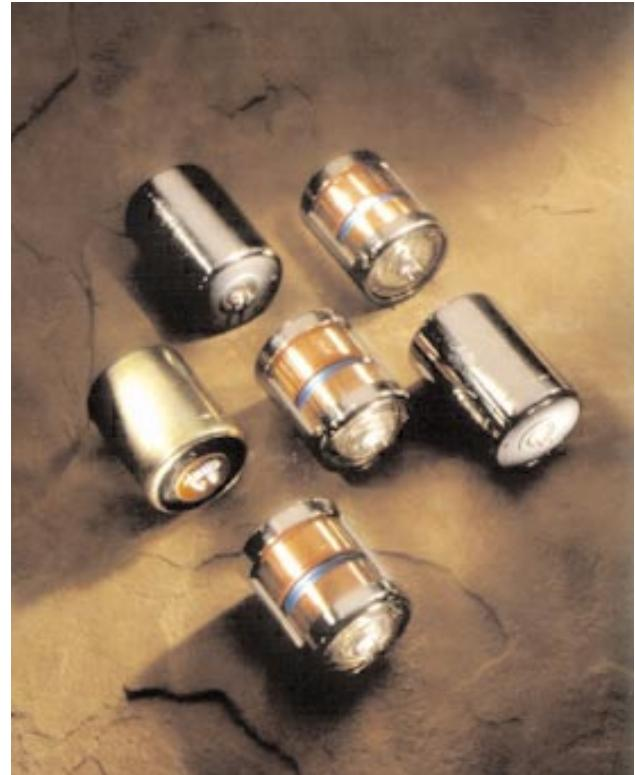
The SM-6 geophone is a long coil travel version of the time proven SM-4 geophone. The extra coil travel offers an advantage for higher tilt requirements and where larger amplitude signals may be encountered, for example in industrial vibration monitoring. A range of natural frequencies is available from 4.5 Hz to 14 Hz, providing choice of the correct geophone for a wide variety of applications.
